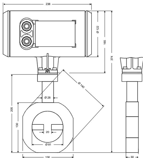
Fig. 5: LiquiSonic Ultrasonic measuring device with immersion and tubular probe
