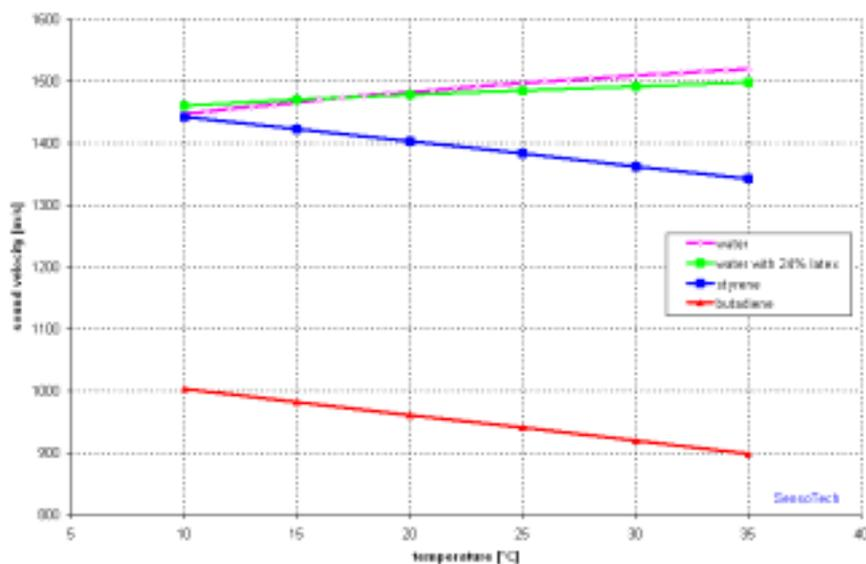
Fig. 1: Sonic velocity of components of butadiene-styrene polymerization.
