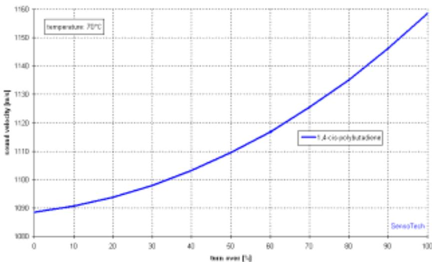
Fig. 3: Materials conversion in butadiene to 1,4-cis-polybutadiene polymerization
