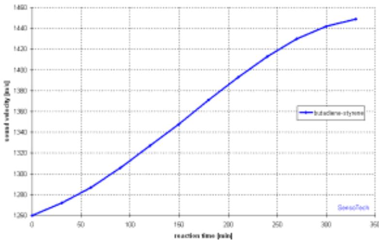
Fig. 2: Variation of sonic velocity during polymerization of butadiene and styrene.
