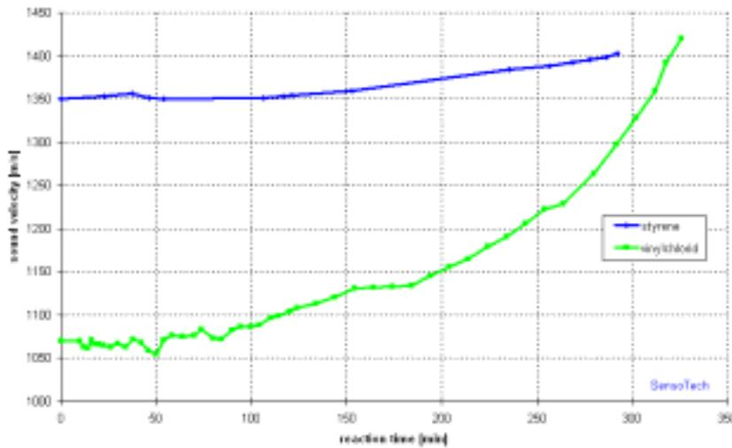
Fig. 4: Sonic velocity during polymerization of vinyl chloride and styrene
