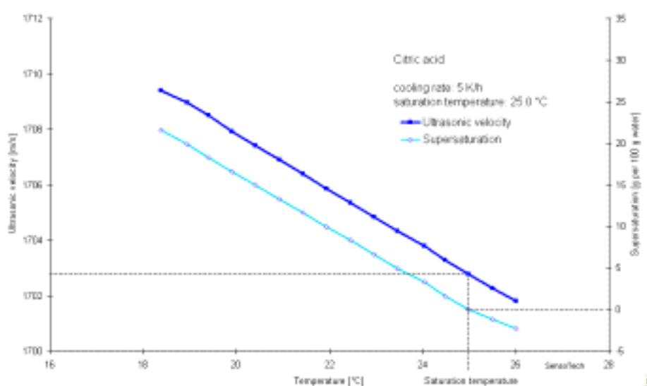
Supersaturation of the solution varies during crystallisation due to crystal growth. Crystal growth reduces the degree of supersaturation. Supersaturation increases again when the temperature of the mother solution is increased or the solvent evaporates.
