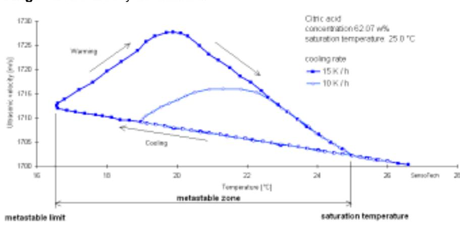
The figure provides an explanation of this effect: if the solution is slowly cooled down, the sound velocity changes at a specific temperature coefficient. From a certain temperature a marked change of the sound velocity can be observed. The relating temperature is the nucleation temperature. If the solution is reheated, its sound velocity curve differs from that obtained during cooling. Both curves meet again at saturation temperature.
