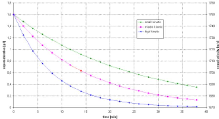
As can be seen, the time curve of sound velocity during crystallisation is identical with that of known supersaturation reduction. The supersaturation reduction curve in the figure below, which was calculated from sound velocity, is compared with the chemical analysis suggested by Tavaré and Chivate [3].
