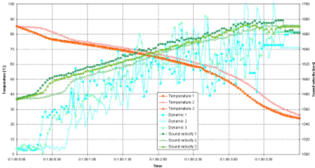
**LiquiSonic®** also calculates the "dynamics" of the current process on the basis of statistical measurement information. The "Dynamic 3" trend shown in the figure signals a clear deviation of this process from the other two processes, and hence facilitates immediate intervention for correcting the process flow.
