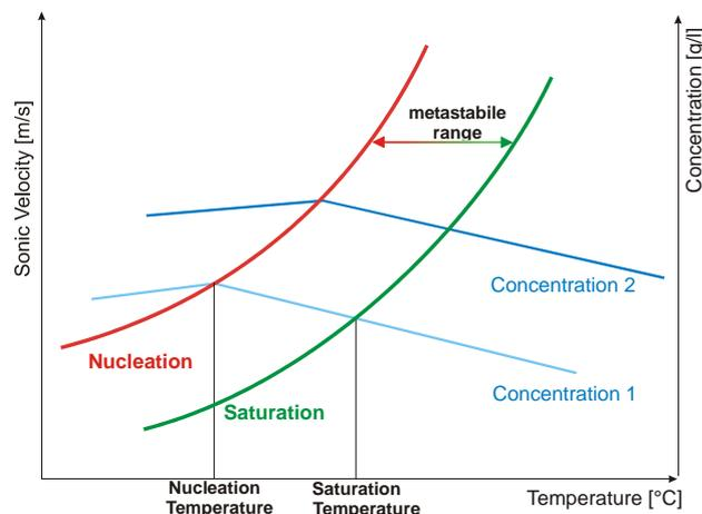
The saturation behaviour depicted in the figure below as a function of concentration, temperature and sound velocity is stored in the **LiquiSonic**® Controller in form of calibration curves.
